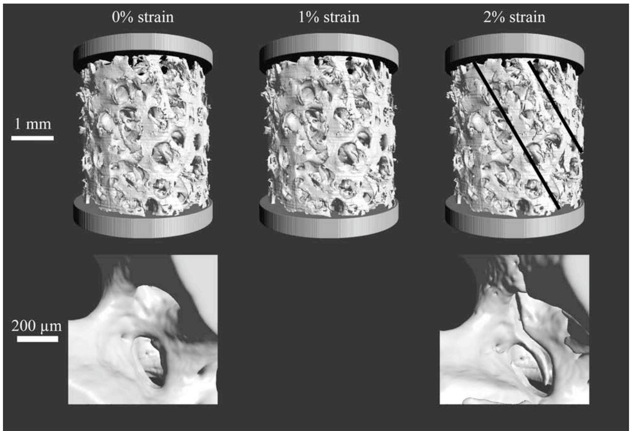
Figure 2: 3D visualization of a detail and the whole non-fatigued bone sample (sample A, Table 1) subjected to IGFA at different compression steps. The sample shows a fracture band going diagonally from the upper left to the lower right through the sample (indicated with the black lines, the failure band is situated in between them). The detail shows the microcrack formation. Data acquired at the MS beamline (SLS) at the photon energy of 20 keV.
