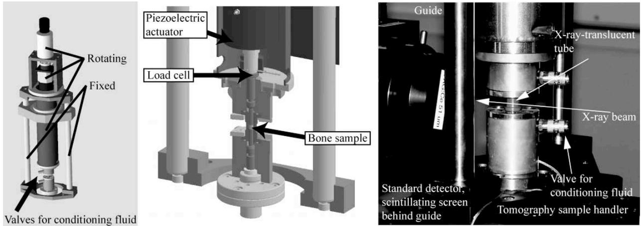
Figure 1: 3D design drawings of the whole IMCSD device (left), and the sample chamber (middle), which is screwed to the actuator housing and the tomography rotation stage. A photograph of the device in operation is given (right).
