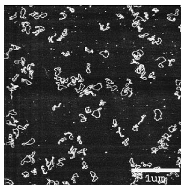
**Figure 5.** AFM image of DNA on mica, scanned in liquid in 25 s using a small (width = 5  $\mu$ m) SiN prototype cantilever with automatically grown EBD tip. DNA line width approximately 20 nm.
