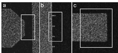
**Figure 2.** The steps of zooming into a cantilever. The framed area has been matched to a reference image by the pattern recognition. (a) Top view of the front part of a cantilever chip, 50 $\times$  magnification. (b) Front edge with cantilever array, 500 $\times$  (c) single cantilever, 10 000 $\times$ .
