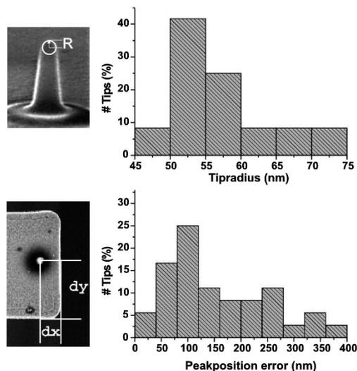
**Figure 4.** Distribution of tip radii and positioning errors on cantilevers.
