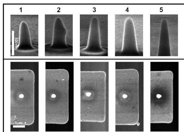
**Figure 3.** SEM micrographs of five finished EBD tips, in side view and top view. The tips were selected randomly from locations across the wafer.
