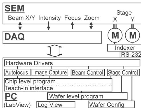
Figure 1. Simplified diagram of the system.
